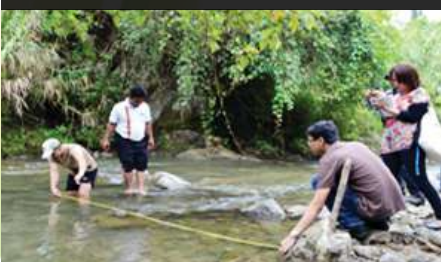
Water discharge measurement and sampling during the field practicum (from one of the tributaries of the Upper Chico River)
